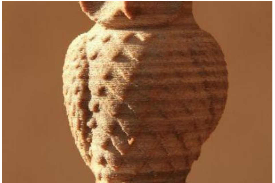
Component printed with Laywoo-D3 composite wood filament
