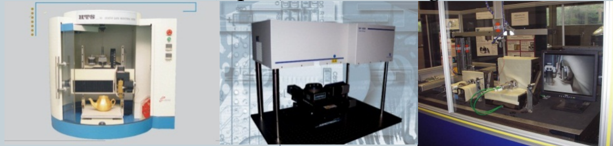
Desktop manufacturing stations: (Left) Typical Rapid Prototyping Machine (Guangzhou Comac); (Middle) SF-100 ELITE Maskless Lithography System (Intelligent Micro Patterning); and (Right) First U.S. Micro-factory at UIUC .
