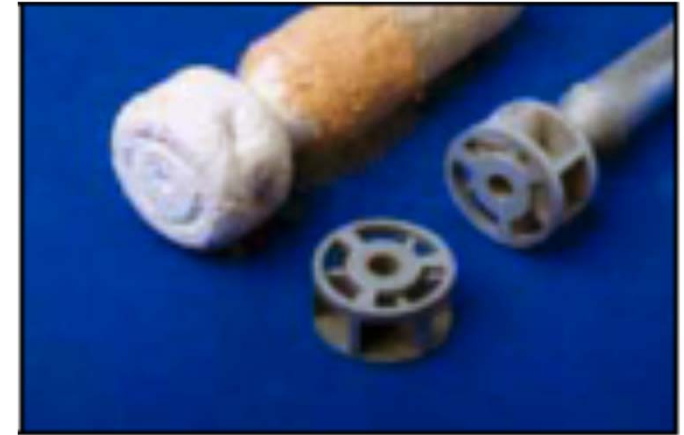
Investment casting shell and cast impeller
