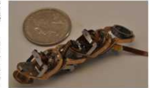
Fig. 2. Four segment Milli-Motein chain with a one centimeter module pitch. The chain folds itself into shapes using our new Electropermanent wobble motor.
