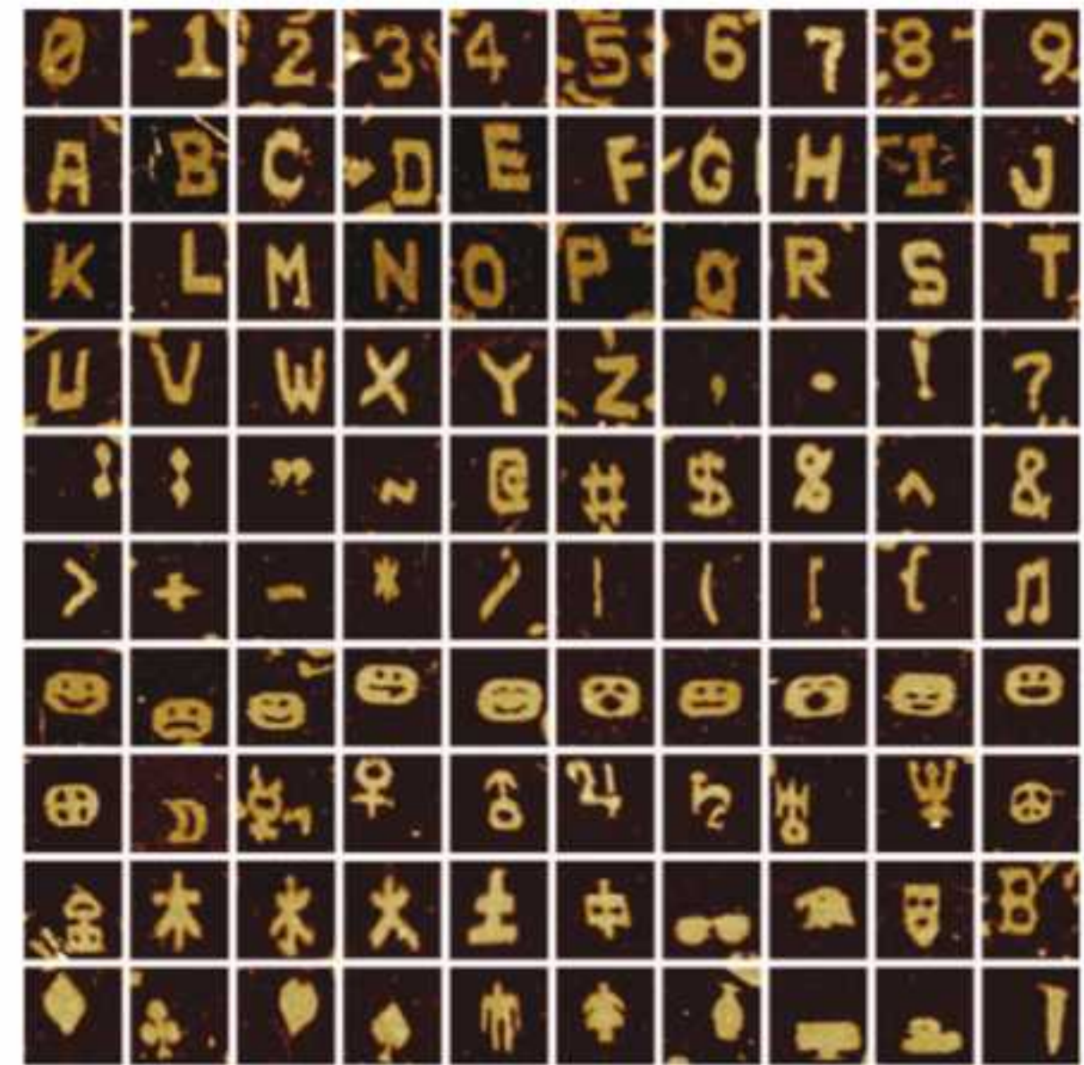
Figure 4 | Complex shapes designed using a molecular canvas. AFM images of 100 distinct shapes, including the 26 capital letters of the Latin alphabet, 10 Arabic numerals, 23 punctuation marks and other standard keyboard symbols, 10 emoticons, 9 astrological symbols, 6 Chinese characters and various miscellaneous symbols. Each image is 150 nm × 150 nm in size.
