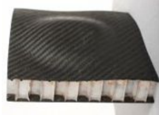
Same construction using proprietary lay-up/curing method. Note smooth outer surface.
